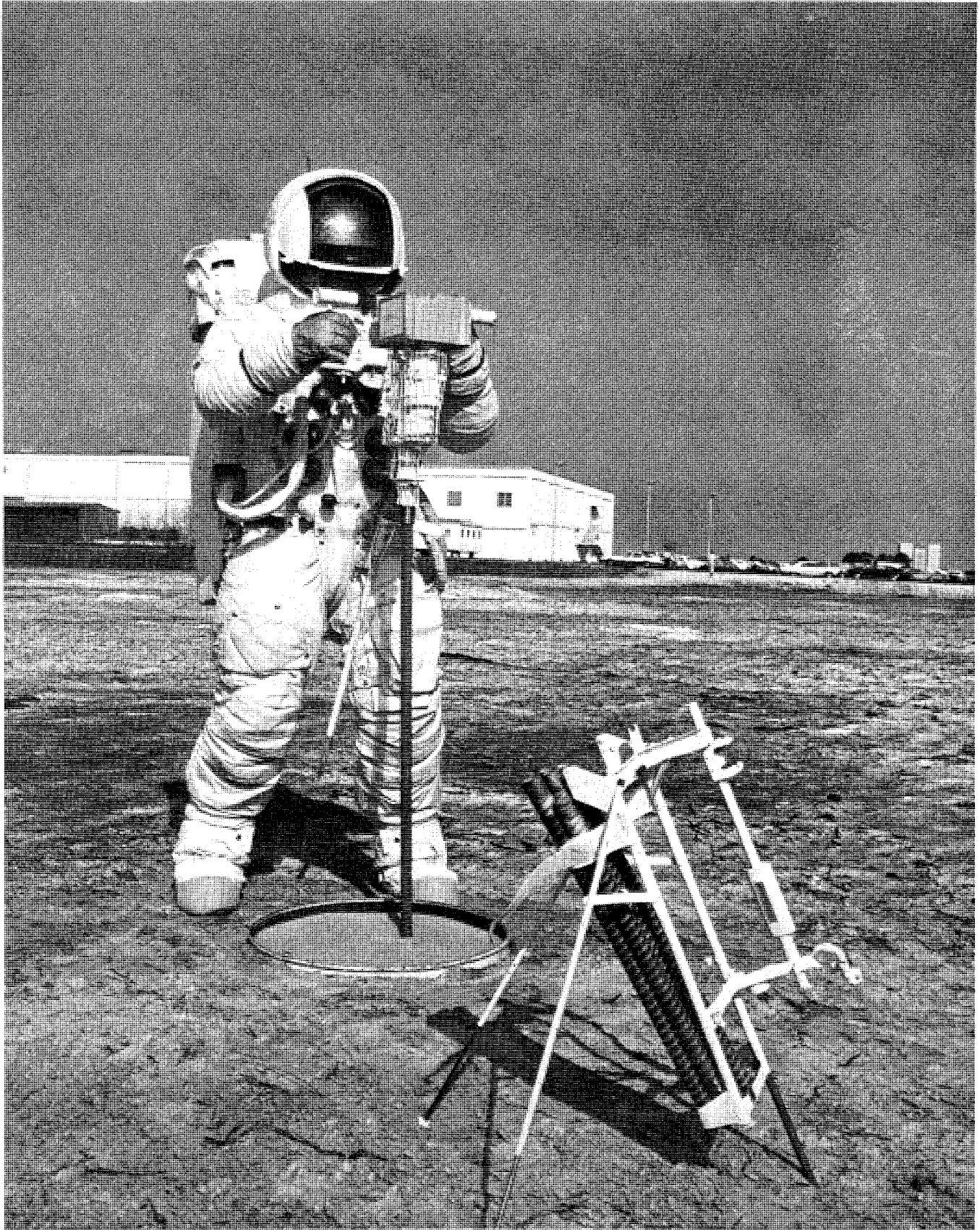
Fig. 20. Apollo Lunar Surface Drill being tested by subject in space suit. The handle, battery, power head and drill stems are visible. A stand containing bore stems is in the foreground (NASA photo S70-29673).
