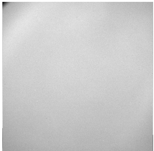
Figure 7. Ratio of dark-corrected sky flat taken with dust cover closed to dark-corrected sky flat taken with dust cover open. Both images acquired on Sol 46. The vignetting at upper left is caused by black tape that was added to the MI dust cover to enable images taken through the cover to be easily recognized.
